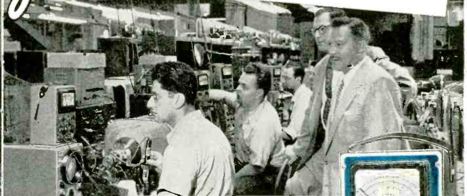
Mr. Al Goldberg, Assistant Chief Engineer of CBS-Columbia, and Harry R. Ashley, President of EICO, inspecting the use of the EICO Model 221 Vacuum Tube Voltmeter and Model HVP-1 High Voltage Probe at the Sweep Frequency Troubleshooting Position on the CBS-Columbia Color Television production lines.
