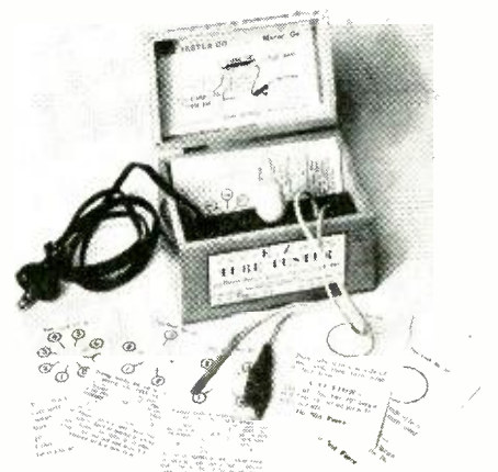
The tester uses 38 punched, coded cards.
